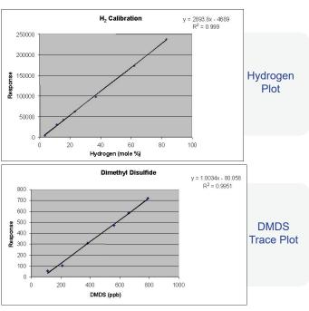
These calibration plots illustrate the linearity of the RTGA in both trace and high level applications.
